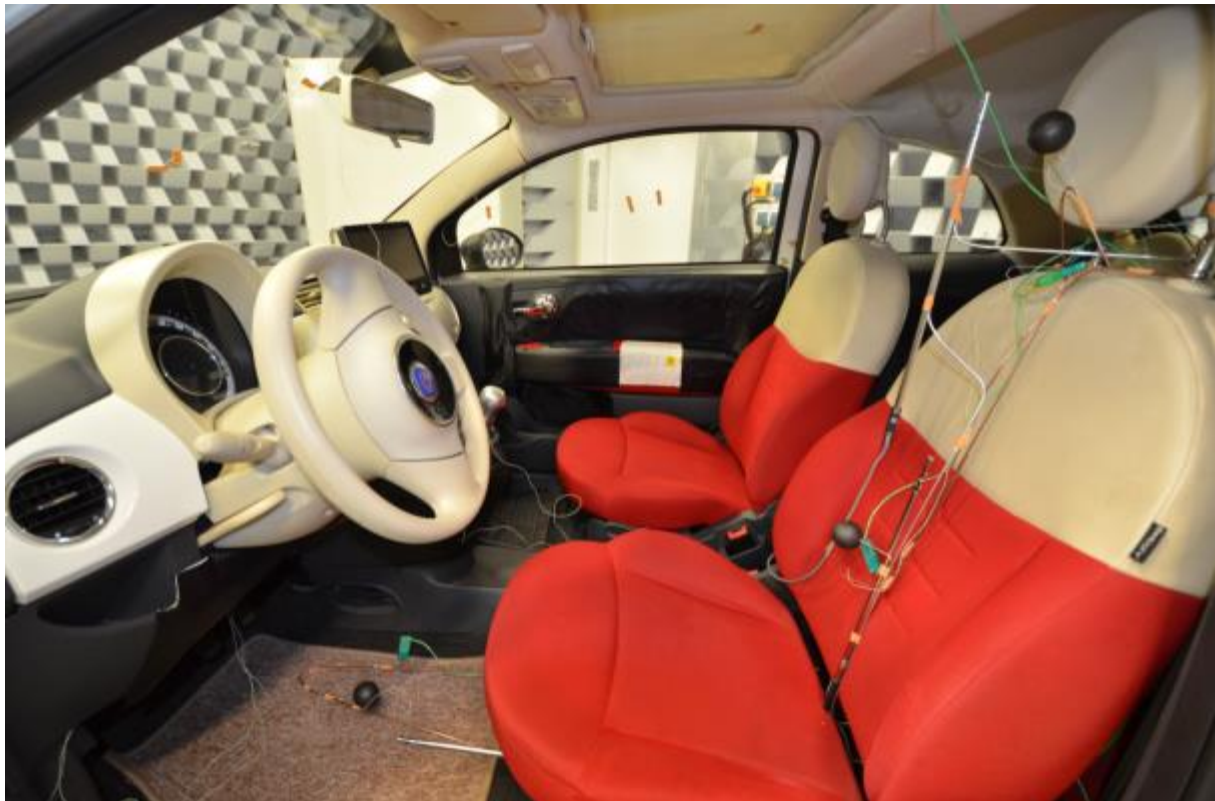
Figure 2-4: Basic sensor system to determine thermal comfort consisting of 3 globe thermometers, 3 air temperature sensors and 3 air velocity sensors (ika)
