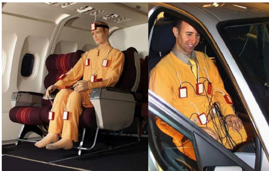
Figure 2-7: Dry heat loss transducer system DRESSMAN by Fraunhofer IBP
