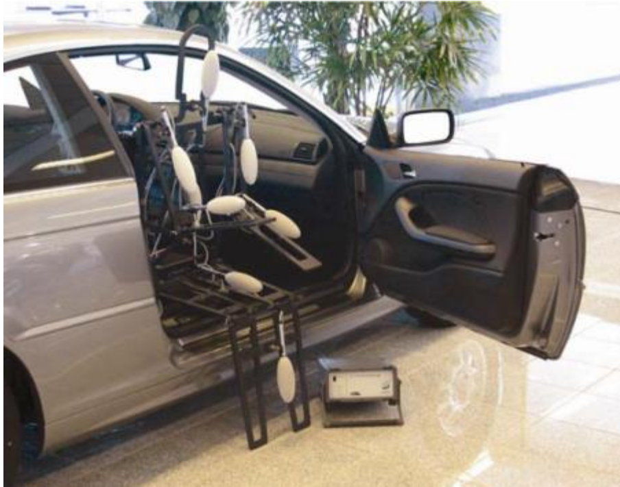
Figure 2-6: Flatman by LumaSense Technologies consisting of MM0057 sensors
